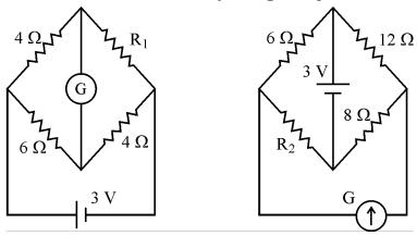
Define the term current sensitivity of a galvanometer. In the circuits shown in the figures, the galvanometer shows no deflection in each case. Find the ratio of  $R_1$  and  $R_2$ .
