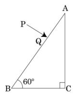
A ray PQ incident normally on the refracting face BA is refracted in the prism BAC made of material of refractive index 1.5. Complete the path of ray through the prism. From which face will the ray emerge? Justify your answer.
