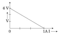
The plot of the variation of potential difference across a combination of three identical cells in series, versus current is shown below. What is the emf and internal resistance of each cell?
