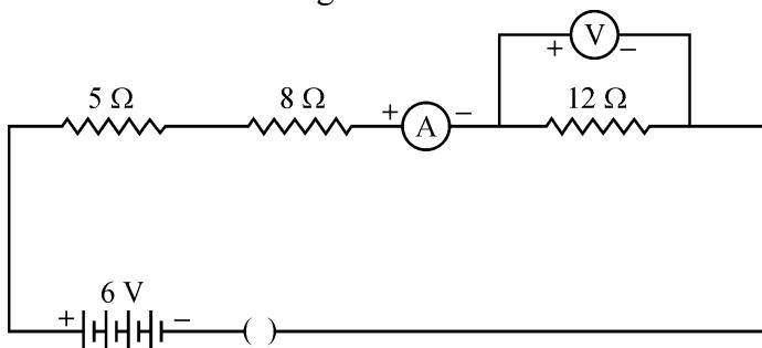
What would be the readings of the ammeter and the voltmeter when key is closed ? Give reason to justify your answers.
